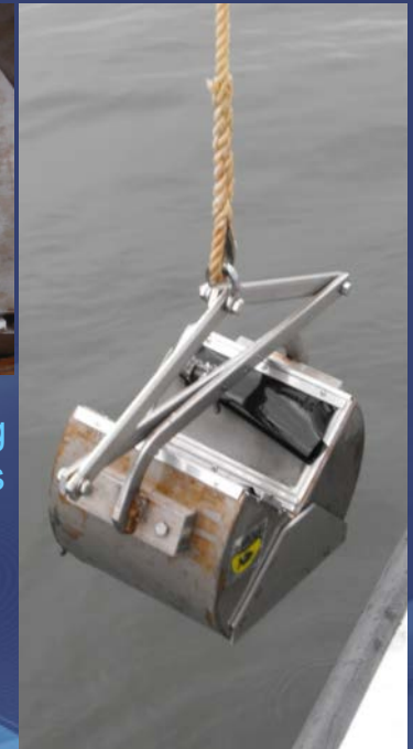
Bottom grab taking sediment samples
