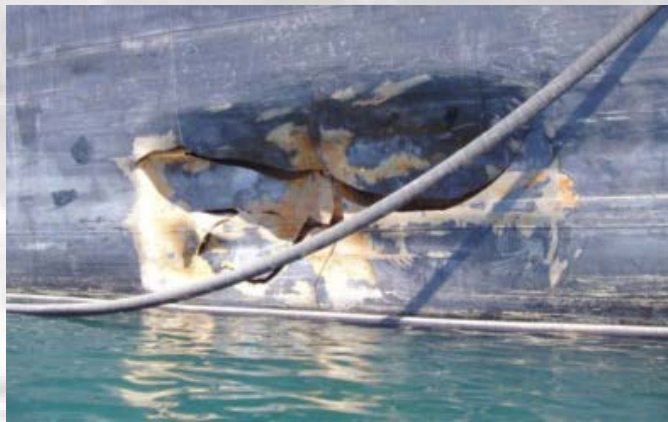
Tanker with Ice damage
